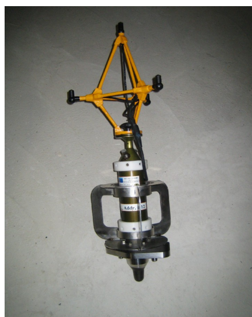
Base unit with the mechanical interface to the male metrology cone
