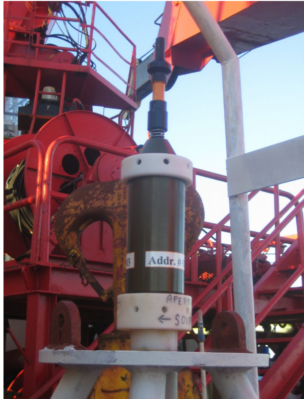
R3000-NG Base with its interferometric frame and R3000 Pointer (Right)
